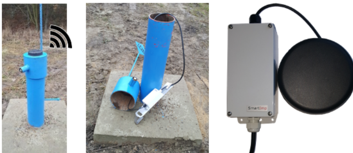
Figure 4 Level measurement with VW probe and data sending with SENSECOM-HP1
