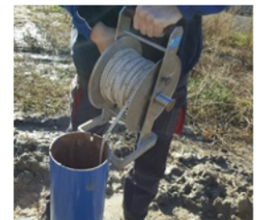
Figure 1 Manual level measurement
