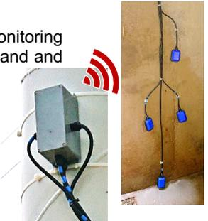
SENSECOM-DI6 for detection of water levels with floats
